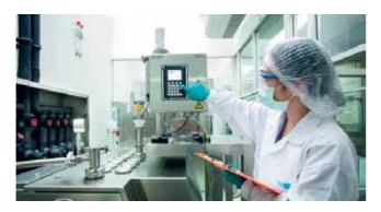
such as compressed tablets, coated tablets and hard gelatin capsules, which are required to be produced in an environmentally controlled clean room (class 100,000 or ISO class 8). The clean room was designed to have smooth surfaces and the corners of the room are set at an angle that can prevent the entrapment and accumulation of dust and germs.
